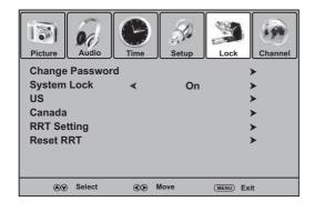
4 Press ▲ or ▼ to highlight RRT Setting, then press ► or ENTER. If the program is broadcast with RRT5 rating information, the rating information is downloaded automatically.
